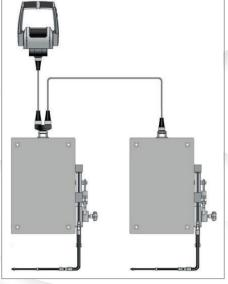
**4500-ME21 Kit Includes:** 2 of Actuator Assembly (4500.A-034039), 1 of Command Lever (4500.C-200005), 2 of Supply Plug (3500.38-00000), 1 of Data Transmission Cable 10 m (3500.33-10000), 1 of Data Transmission Cable 3 m (3500.33-03000), 1 of CANBus T-splitter (N-85E010003), 2 of Actuator to Transmission Cable (3500.46-03000)
